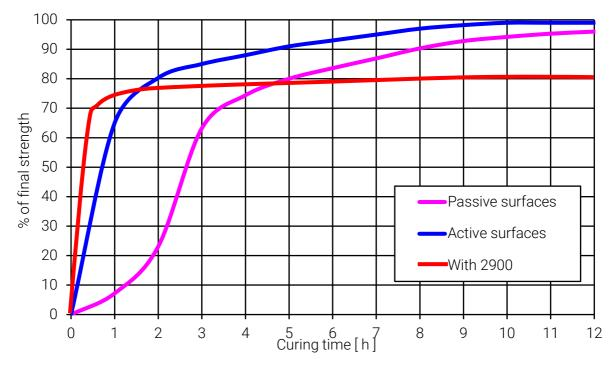
Note: The use of the activator reduces the final strength of the adhesive used by up to 20% compared to the ideal values.
